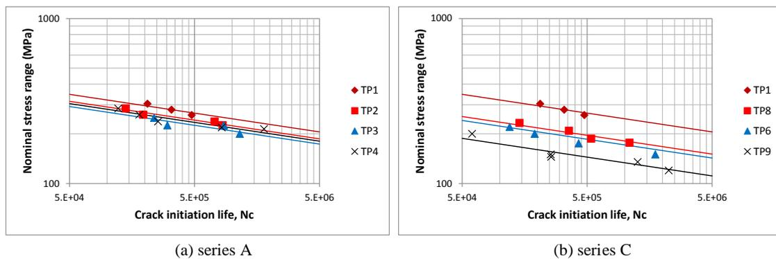
Fig.6 Relation between nominal stress and crack initiation life (series A & C)
