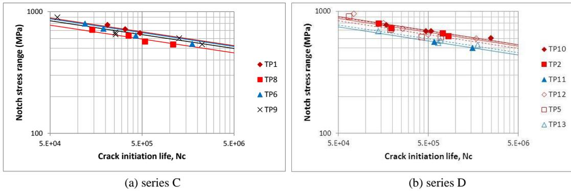
Fig.7 Relation between notch stress and crack initiation life (series C & D)
