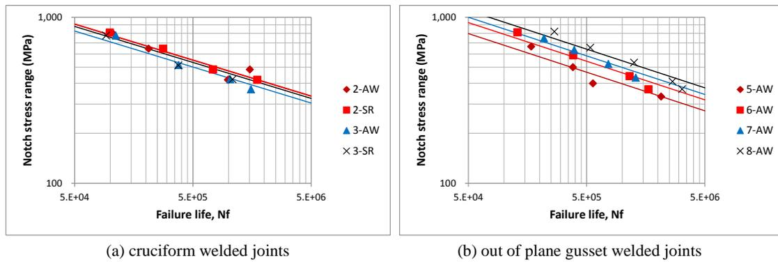
Fig. 9 Relation between notch stress and failure life
