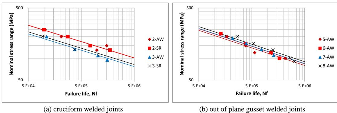
Fig.8 Relation between nominal stress and failure life
