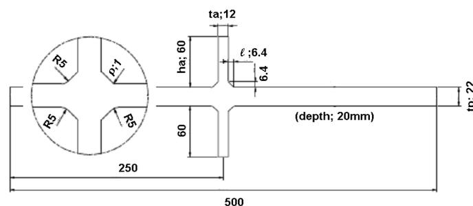
Fig. 1 Example of test specimen in fundamental experiment
