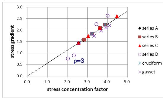
Fig. 5 Relation between stress concentration factor and stress gradient.
