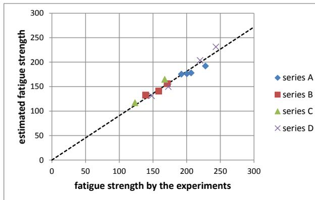
Fig.12 Relationship between the fatigue strength estimated by the Siebel's diagram and the fatigue strength calculated by the S-N curve derived from the fatigue tests
