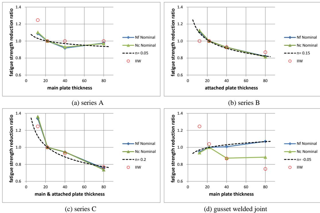
Fig.10 Fatigue strength reduction due to thickness effect
