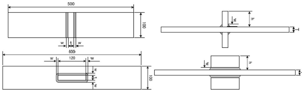
Fig. 2 Test Specimen in basic welded joint experiments
