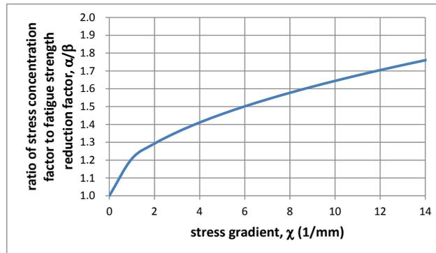
Fig.11 Correlation between the stress gradient ( $\chi$ ) and the ratio of stress concentration factor to fatigue strength reduction factor ( $\alpha/\beta$ ) for the material used in the fundamental experiments derived from Siebel's diagram
